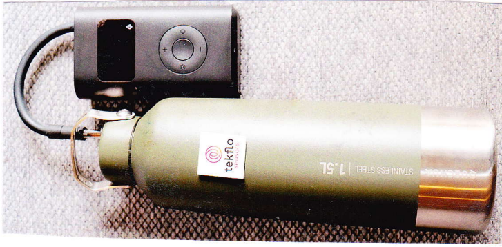
nanoTek air canister with pressure connector and gauge at the top. Max. pressure 300 psig (29.7 bar g) Stainless steel AISI 316 Weight 2.4 kg (5.3 lb lb)
